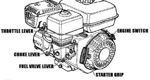
This engine is equipped with an *Oil Alert System* which is designed to prevent engine damage caused by an insufficient amount of oil in the crankcase. Before the engine can fall below a safe limit, the *Oil Alert System* will automatically stop the engine (the engine switch will remain in the ON position). The *Oil Alert System* is sensitive to the engine being operated at an incline. Operate ventilator within the design limits of the engine tilt lever.
