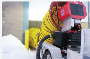
SVU outlet duct for directing positive pressure air
